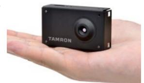
Shutterless Far-Infrared Camera Module
